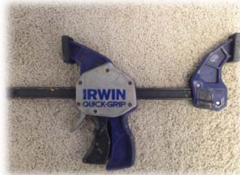
There are some adjustable carpenter C-clamps which have a reversible end – so that instead of only squeezing parts together, it would push things apart. Pick a size which will fit in appropriate spots on your engine. The cushion pads on the clamp help to keep it in position – and, now you have an extra hand to hold the belt tension (per engine mfg. recommendation), while you work the wrenches to finish the job.
